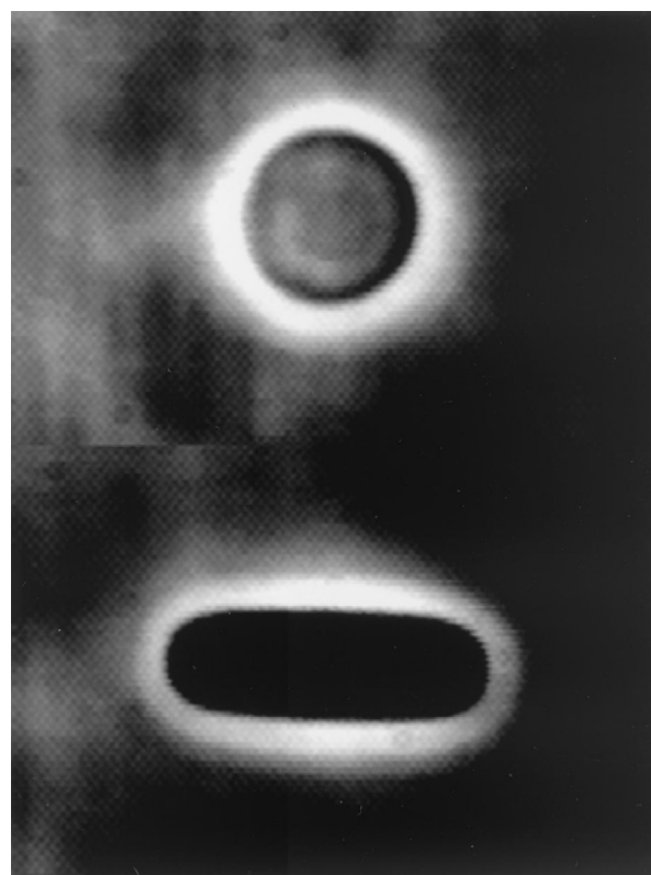
FIGURE 12 An example of an RBC stretched beyond the linear regime. The top part shows the undeformed cell trapped at 5 mW with a radius \rho = 3.36 \pm 0.05 \mu\text{m} . In the lower part, the cell is stretched with a peak stress \sigma_0 \approx 2.55 \pm 0.10 \text{ Nm}^{-2} to \rho = 6.13 \pm 0.05 \mu\text{m} along the beam axis, an increase of 82 \pm 3\% . After reducing the power, the cell returned to its original shape.
